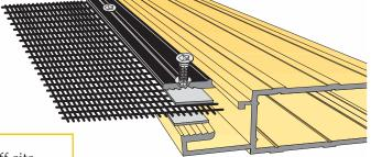
right through mesh and frame - for unbeatable strength
